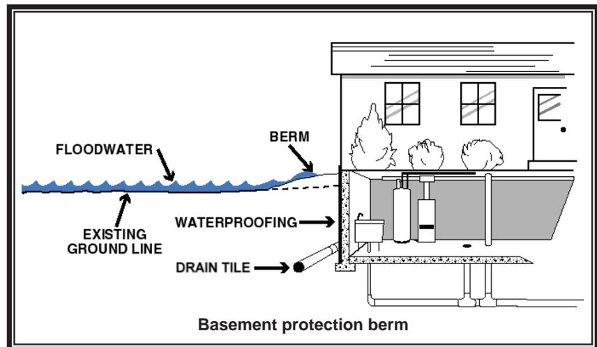
Sump pumps cannot keep up with surface water. If you have sandy or permeable soil, you should consult an engineer or soils expert to ensure that the berm will extend far enough away from the walls. **Don't forget: filling or grading in your yard requires a permit.**
