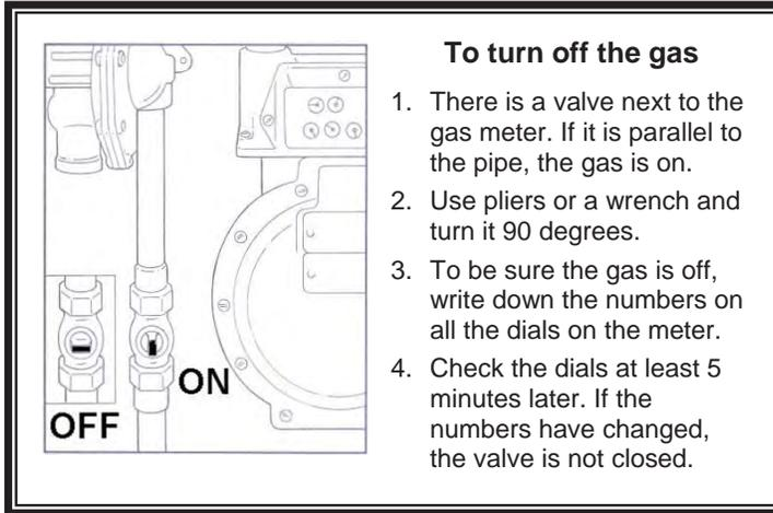
Most gas meter valves have a hole in the handle that lines up with a hole in the valve body when the gas is shut off. This hole is used by the gas company to lock or seal the valve closed when the building is vacant. When the holes are lined up, you know that the gas supply has been shut off. If you have any doubts, play it safe and call your gas company.
