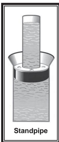
**Standpipe:** A standpipe is an inexpensive alternative to a floor drain plug. When the sewer backs up, the water moves up the pipe. If properly installed, water pressure cannot build up to blow a standpipe out of the floor drain. The system works unless the backup is so deep that it goes over the top of the pipe.
