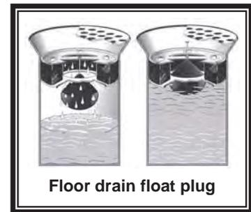
One variation is a plug with a float. It allows water to drain out of the basement (see illustration, left side). When the sewer backs up, the float rises and plugs the drain (see illustration, right side). A float plug permanently installed will not interfere with the floor drain's normal operation.
