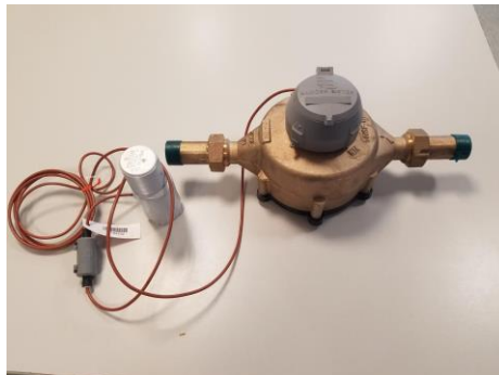
Meter with Cellular Head
